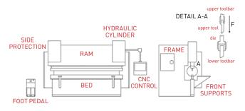
The bending press is described by parameters that can be classified as follows:
